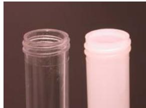
**15 ml Polycarbonate Vials** are large, sturdy vials used for homogenizing large samples or pooled samples. Up to 15 corn kernels or 3 gm of tissue can be homogenized in these large vials. These vials can be chilled in liquid nitrogen and used directly for cryogenic homogenization.
